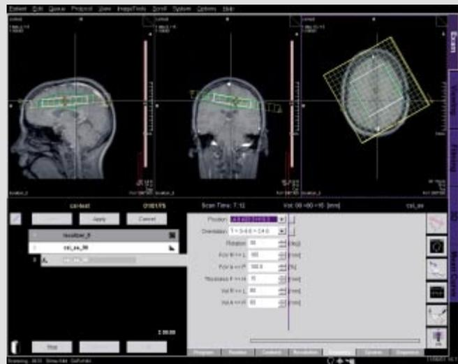
Single Voxel Spectroscopy for proton spectroscopy can be performed using the CP Head Array for image acquisition. Automatic adjustment, measurement and evaluation protocols permit largely automatic spectroscopy measurements.
